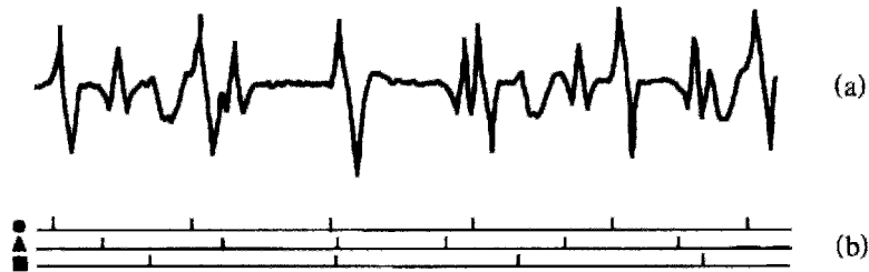
FIGURE 1.7 (a) An EMG signal containing three different waveform complexes. (b) Three impulse trains showing the times of occurrence of these complexes. [Adapted from Guiheneuc, fig. 1, with permission]
