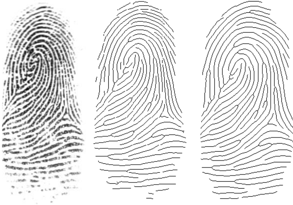
Figure 4.10: Example 2: application of the proposed frequency distortion removal enhancement technique on fingerprint image and its comparison with Gabor Enhancement, (a) Fingerprint 2, (b) Thinned Image based on Gabor Enhancement [30], (c) Thinned Image based on our proposed Enhancement technique
