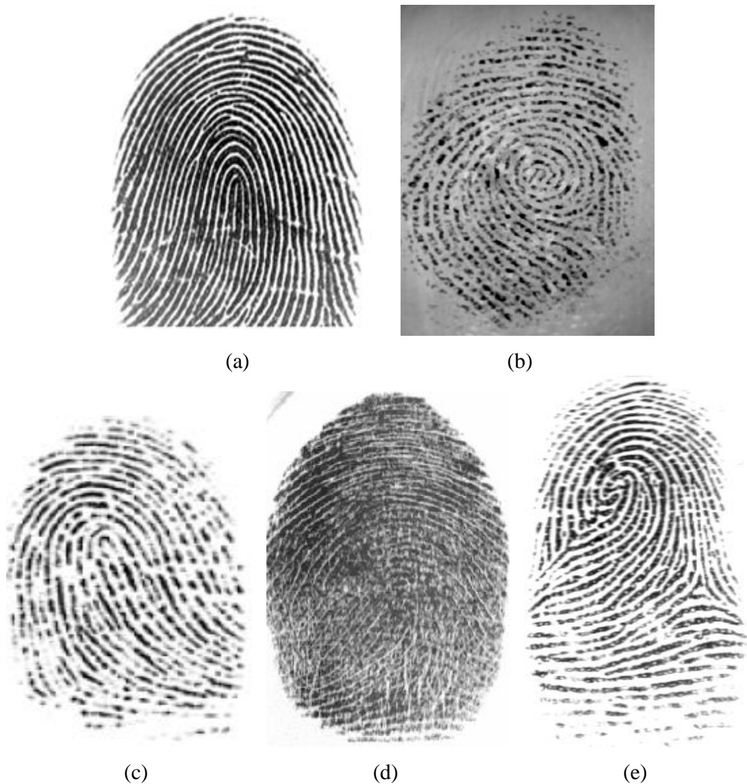
Figure 1.8: An example of different fingerprint images with varying quality. (a) Good quality image, (b) & (c) Fingerprint with low contrast and broken ridges, (d) Low quality fingerprint image with insufficient distinction between ridges and valleys, (e) Fingerprint having non-uniform inter-ridge separation
