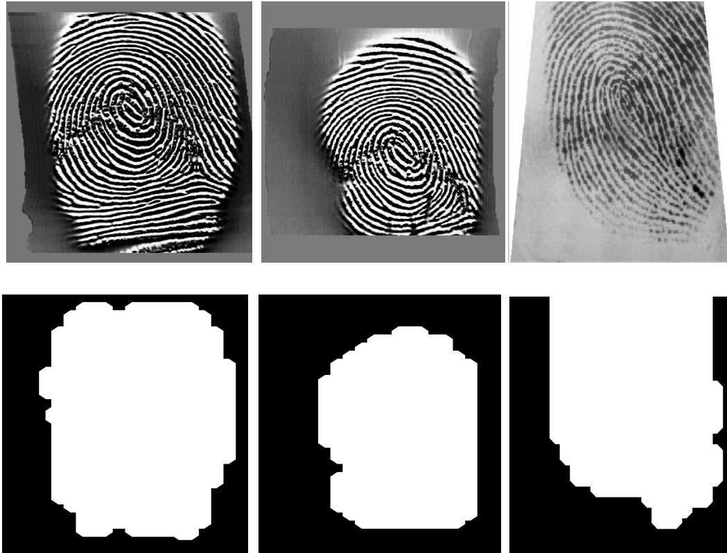
Figure 2.3: Images segmented based on intensity variance based method
