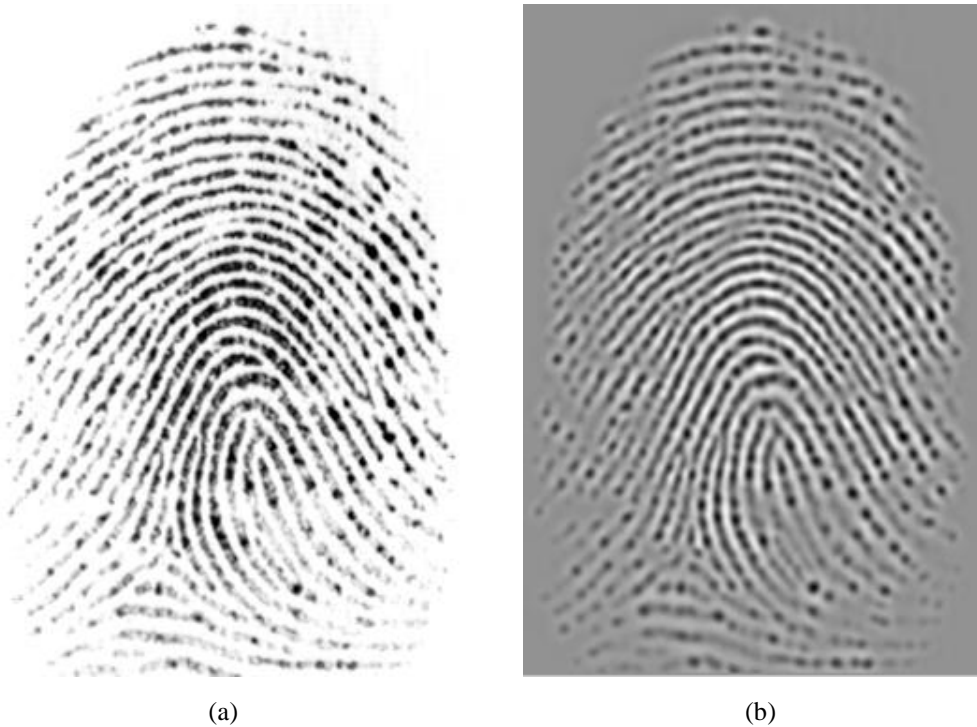
Figure 3.5: Enhanced fingerprint images after proposed directional smoothing method, (a) Fingerprint image 14_7.tif, (b) Unified band-pass enhanced image.
