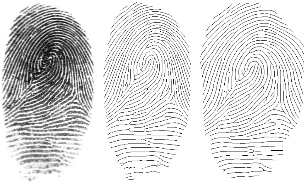
Figure 4.9: Example 1: application of the proposed frequency distortion removal enhancement technique on fingerprint image and its comparison with Gabor Enhancement, (a) Fingerprint 1, (b) Thinned Image based on Gabor Enhancement [30], (c) Thinned Image based on our proposed Enhancement technique
