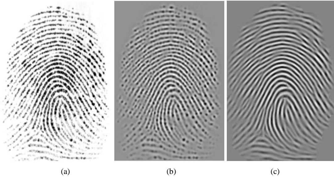
Figure 3.7: Enhanced fingerprint images after proposed directional smoothing method, (a) Fingerprint image 14_7.tif, (b) Unified band-pass enhanced image, (c) Enhanced images after directional smoothing
