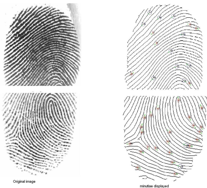
Figure 2.25: Results of Minutia Extraction after False Minutiae Removal
