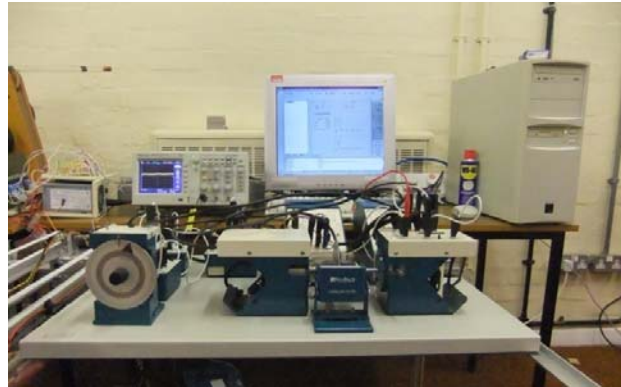
Figure 3.11: The DC Motor and dSPACE Setup
