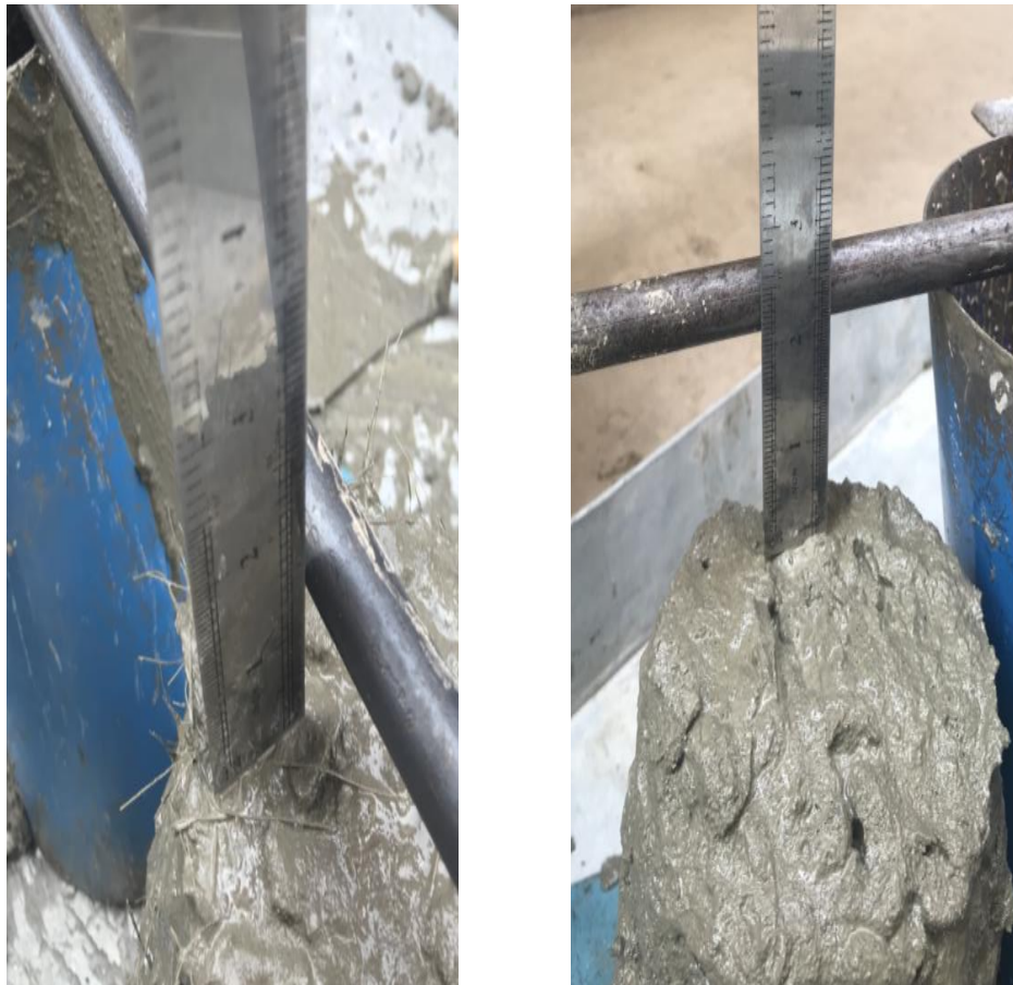
FIGURE 3.1: Slump of JFRC and PC
