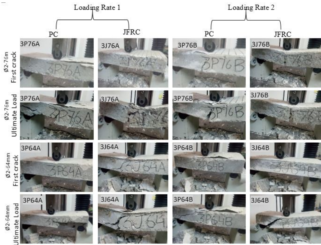
FIGURE 4.5: Crack propagation of PC and JFRC specimens with changing shear rebars
