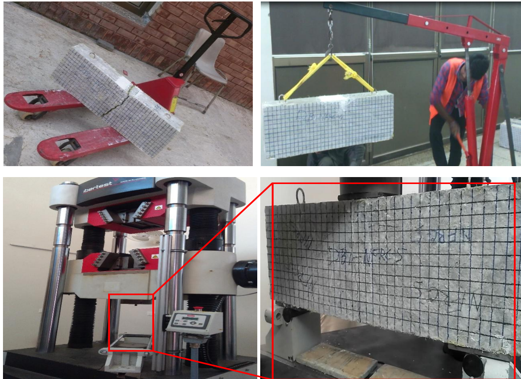
FIGURE 3.4: a) Weight lifter, b) Small-scale hydraulic crane, c) STM, d) Placed Sample in STM
