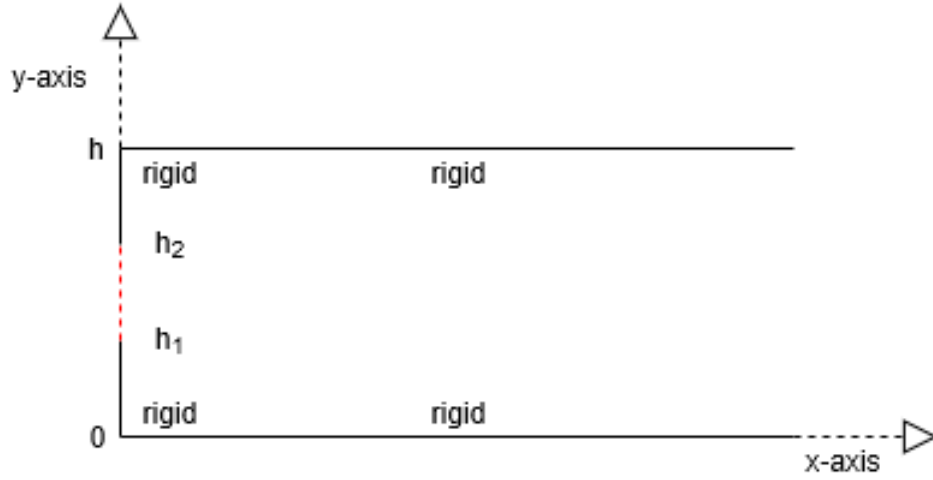
Figure 3.2: The physical configuration of semi-infinite duct
