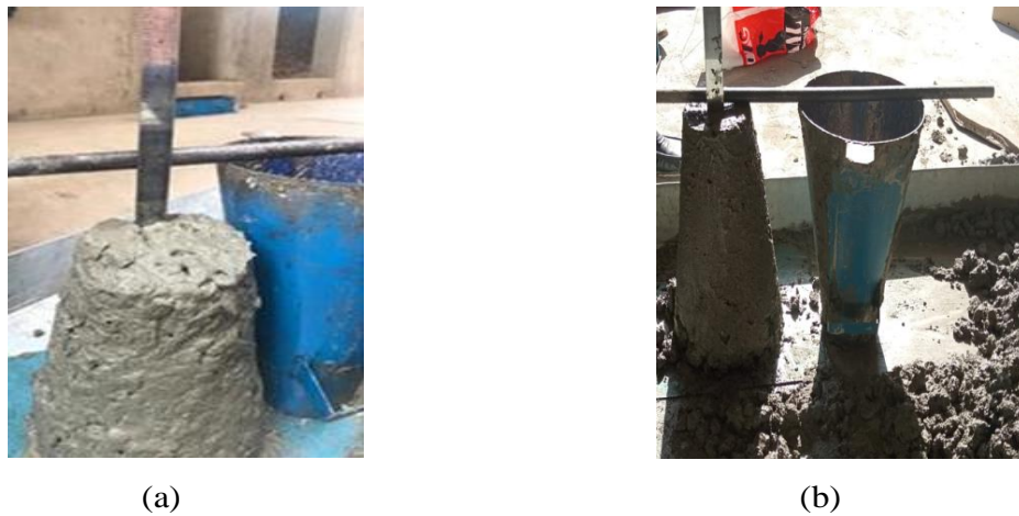
FIGURE 3.3: Slump test a) For PC b) For JFRC.
