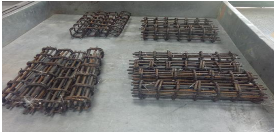
FIGURE 3.2: Steel reinforcement for prototype piers
