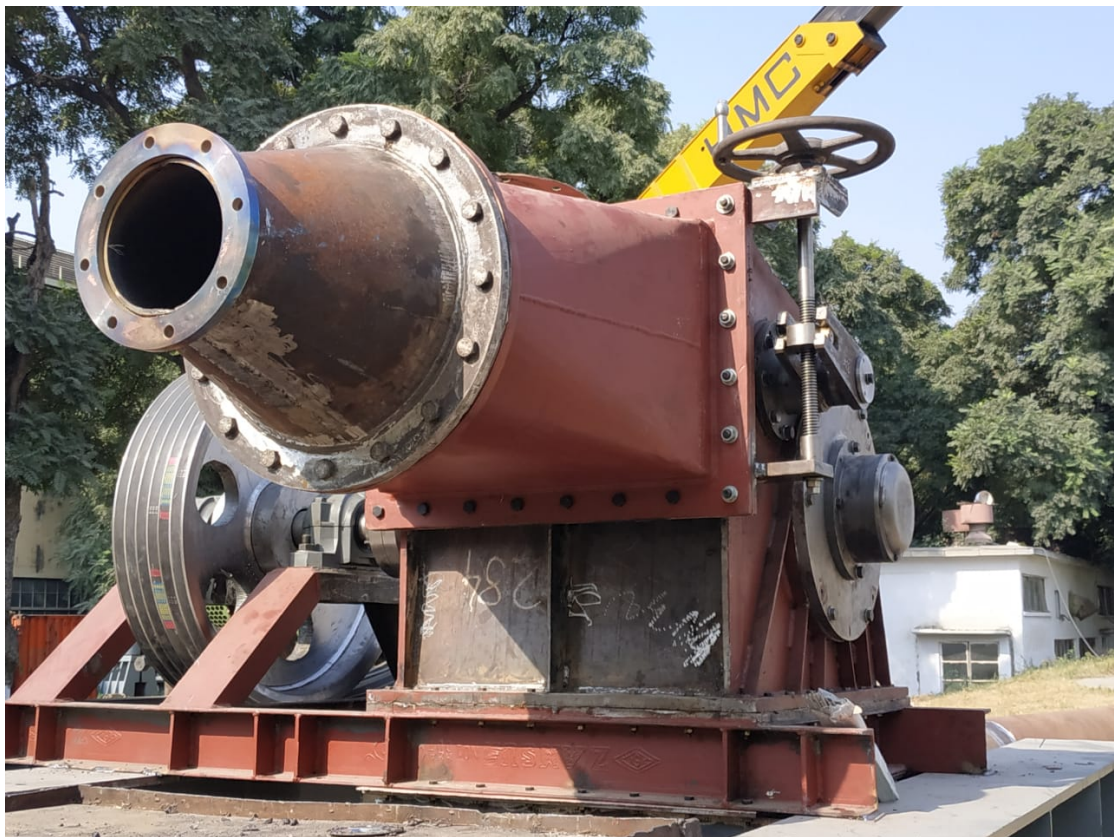
FIGURE 6.1: Cross-flow turbine setup for performance analysis.
