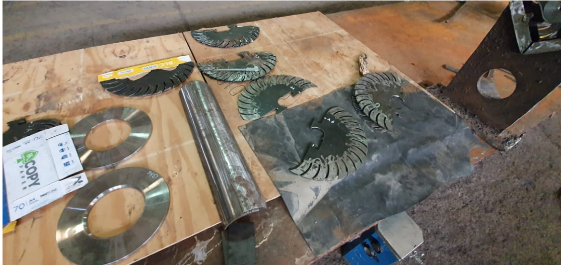
FIGURE 4.20: Components of rotor assembly after machining.
