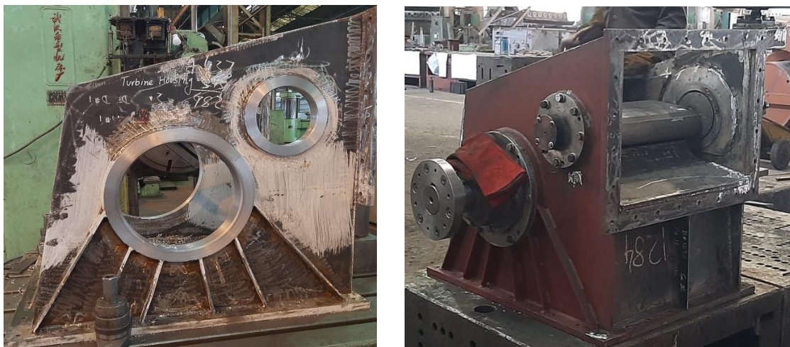
FIGURE 4.4: Turbine housing after machining and arrangement of components inside.
