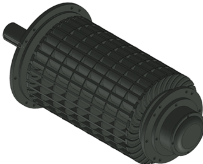
FIGURE 4.12: Turbine rotor assembly solid works model.
