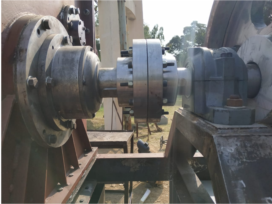
FIGURE 6.2: Turbine pulley and rotor shaft coupling.
