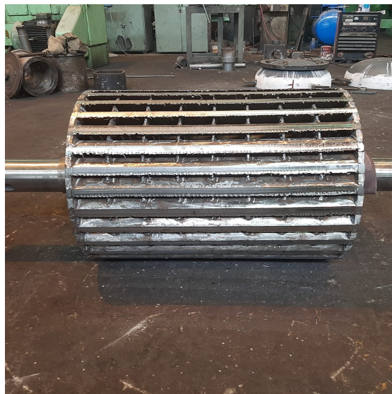
FIGURE 4.23: Turbine rotor after fabrication.
