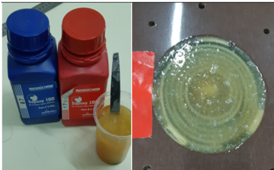
FIGURE 3.5: Epoxy resin and coil fixation process in fiber wood
