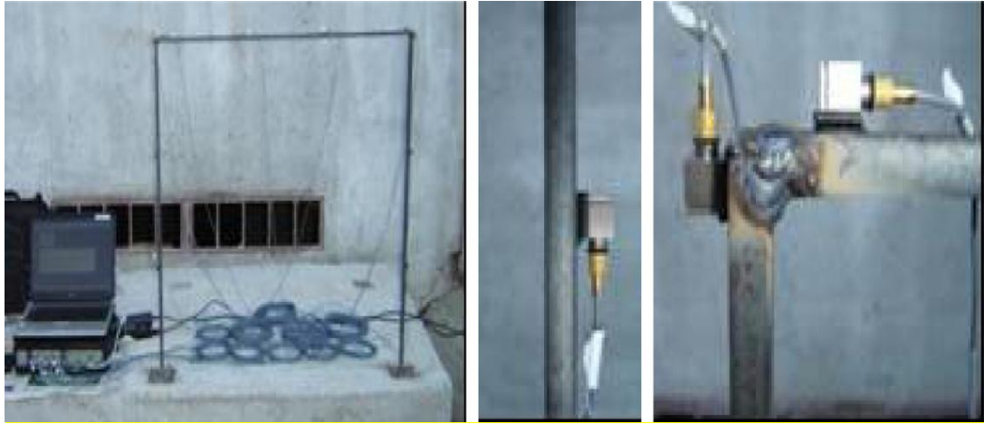
FIGURE 2.3: Studied two-dimensional steel frame [8]
