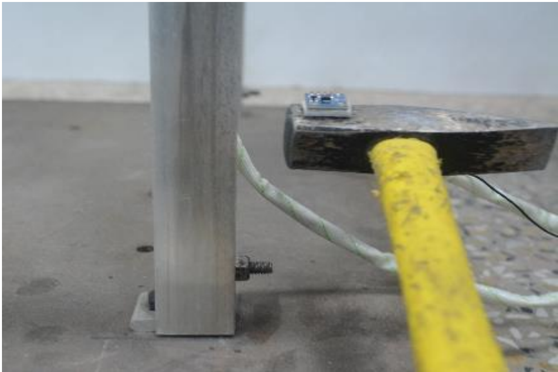
FIGURE 3.2: Calibrated hammer used for the application of impact load
