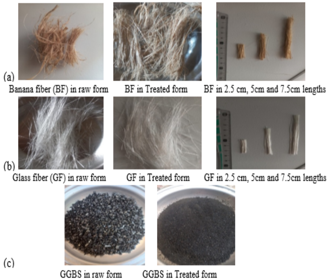
FIGURE 3.1: Images of (a) Banana fiber (b) Glass fiber (c) GGBS in their treated and untreated variants
