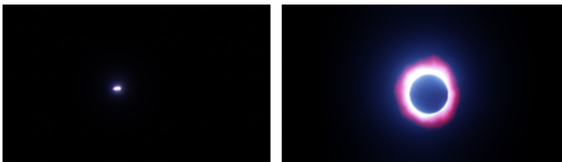
FIGURE 4.4: Increasing size of plume (frame 1 showing a small plume size (left) and frame 15 showing a Large plume (right) eluded by missile body from the center)
