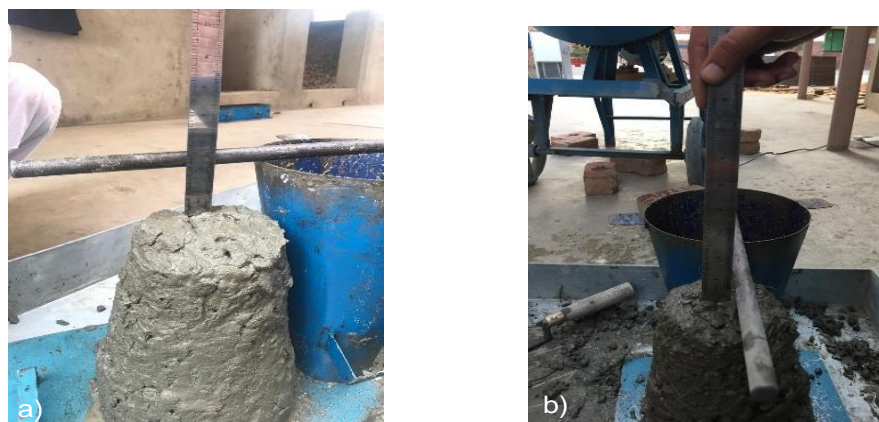
FIGURE 3.3: Slump (a) PC and (b) JFC
