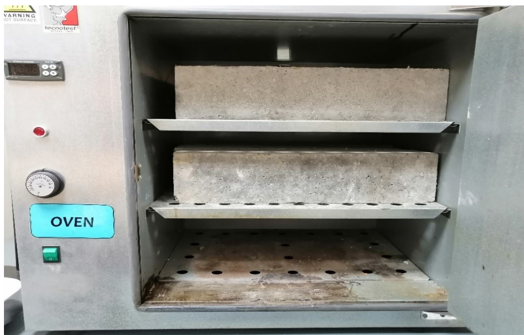
FIGURE 3.4: Drying Samples in Oven for Water Absorption and Mass Loss Test
