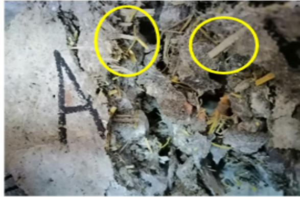
Pull out of wheat straw fibers
