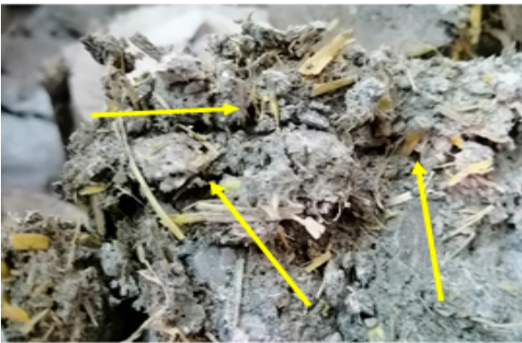
Bond of fibers with surrounding matrix
