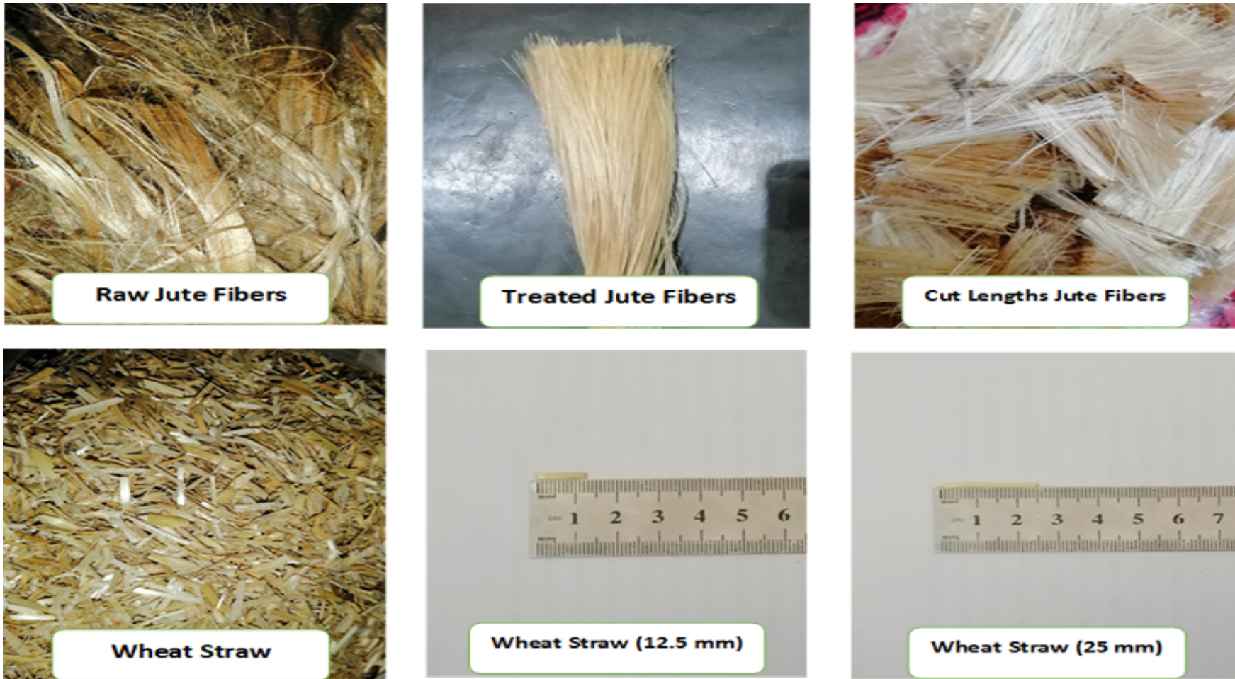
FIGURE 3.1: Images of Jute Fibers (Raw, Treated, Cut Lengths Used) and Wheat Straw
