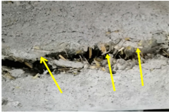
Bridging effect of fibers
