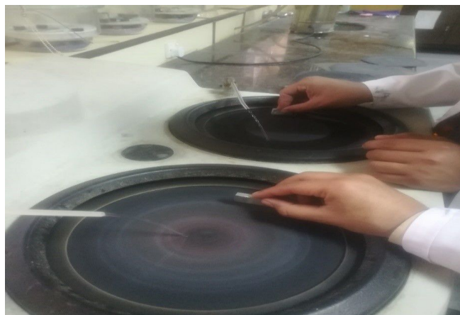
FIGURE 3.20: Grinding and polishing of the specimens
