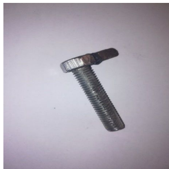
FIGURE 3.8: M12 bolt after welding with rod
