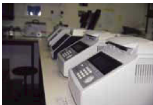
Figure 17.5 DNA thermal cyclers used for PCR amplification of DNA
