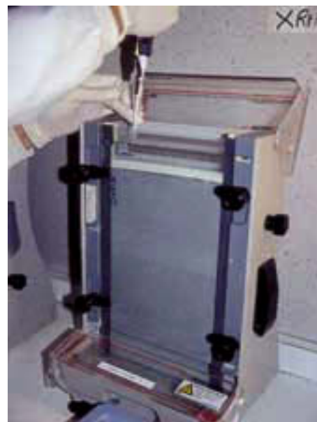
Figure 17.11 Loading PCR-amplified DNA onto an SSCP/heteroduplex gel
