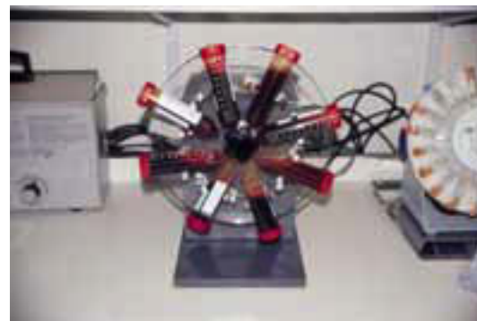
Figure 17.2 Blood samples undergoing lysis during DNA extraction. As little as 30 \mu l of whole blood can provide sufficient DNA for a simple PCR-based analysis
