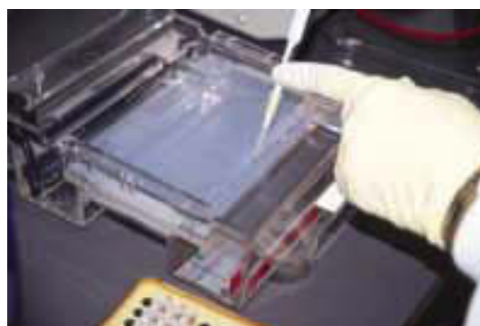
Figure 17.7 PCR amplified DNA being loaded onto an agarose gel before electrophoresis
