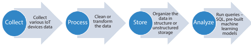
Figure 2.3 IoT data analytics. Adapted from AWS IoT [3].
