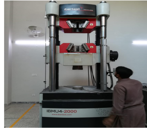
FIGURE 3.3: Testing of beam-lets with rebars: (a) representation diagram, and (b) testing setup
