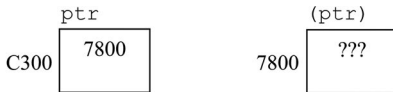
#1: MyType pointer variable 'ptr' allocated on stack MyType object allocated on heap: address placed in ptr
