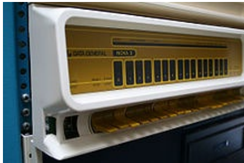
Figure 2.5. On a data general nova 3 from the mid-1970s, there are switches for manual input.
