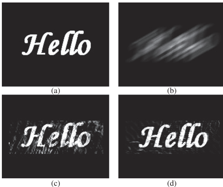
Fig. 23.1. Restoration of Hello image. (a) True image, (b) motion blurred with L = 60 , \theta = 30 , (c) restored with IBD in 126 iterations (PSNR=17.13 dB), (d) restored with IIBID in 50 iterations (PSNR=20.57 dB)
