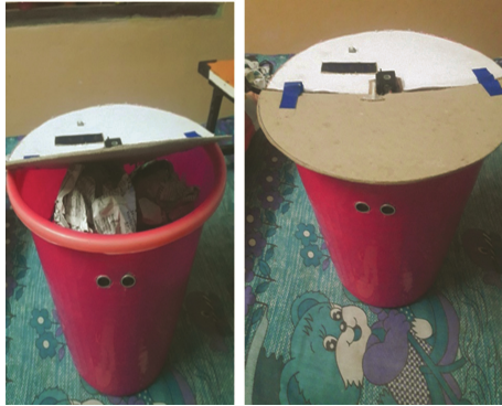
FIGURE 9.2 Witty Bin with its sensor-enabled lid (open and close positions).
