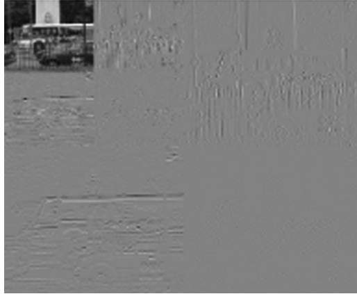
Fig. 15.2 Video frame after two-level wavelet transformation
