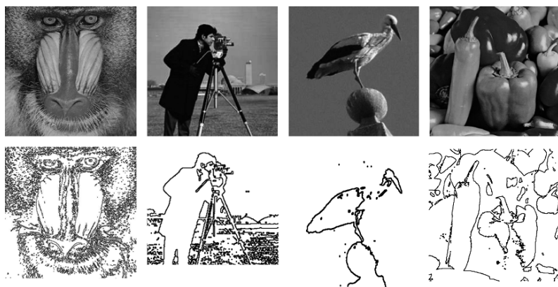
Fig. 16.4 Test images and edge detection results
