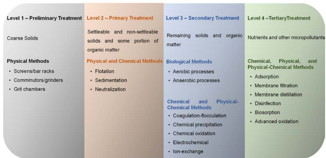
FIG. 7.1 Characteristics of the compounds and treatment methods involved in the different levels of wastewater treatment. Based on A. Ullah, S. Hussain, A. Wasim, M. Jahanzaib, Development of a decision support system for the selection of wastewater treatment technologies , Sci. Total Environ. 731 (2020) 139158.
