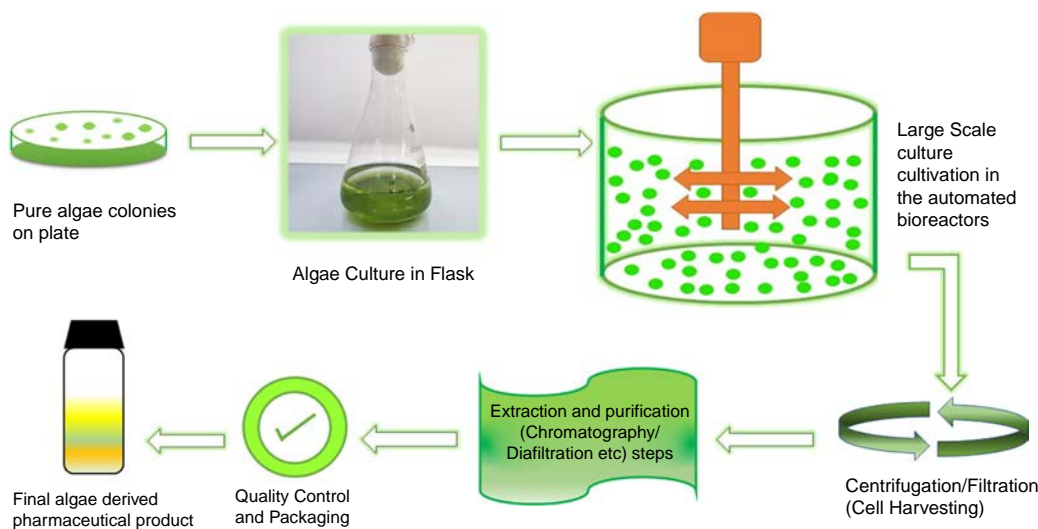
FIG. 14.1 Steps involved in bioprocessing for biopharmaceuticals.
