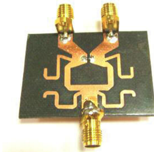
FIGURE 3.1: The Realized Dual Band Wilkinson Power Divider [14].
