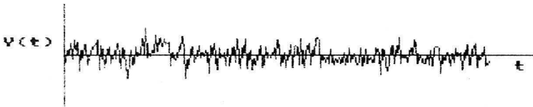
Figure 2.4. A random white noise signal having a Gaussian amplitude probability distribution (see §3.1.1) and a uniform spectral density distribution (see §3.2.2). Note the relatively rare occurrence of extreme values, compared with the signal in figure 2.3.
