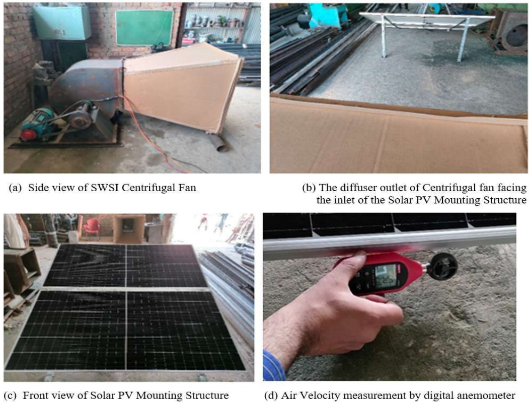
FIGURE 3.5: Configuration of Centrifugal Fan Setup
