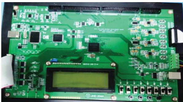
Figure 6.5 SPARTAN6 FPGA controller.
