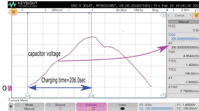
Figure 6.9 Supercapacitor total charging time at constant input voltage of 70 V and 75% duty cycle.
