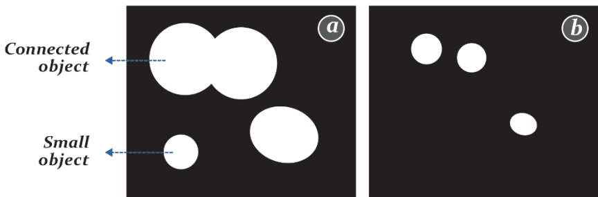
Figure 12.4 (a) Connected and small objects. (b) Erosion of the image in (a) where the disk structuring element is so large that small objects are lost [10] / with permission of SPIE.
