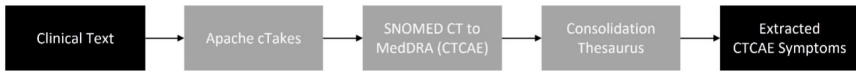
Fig. 1. A natural language processing pipeline, which can be used for extracting CTCAE symptoms from radiation oncology on-treatment visit notes with high accuracy.
