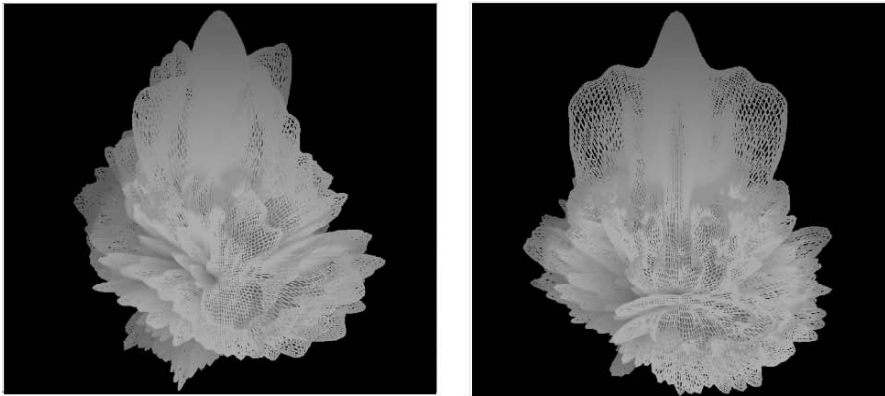
Fig. 2.9 3D beam patterns of the square FZPs: vertical orientation ( left ) and diagonal orientation ( right )
