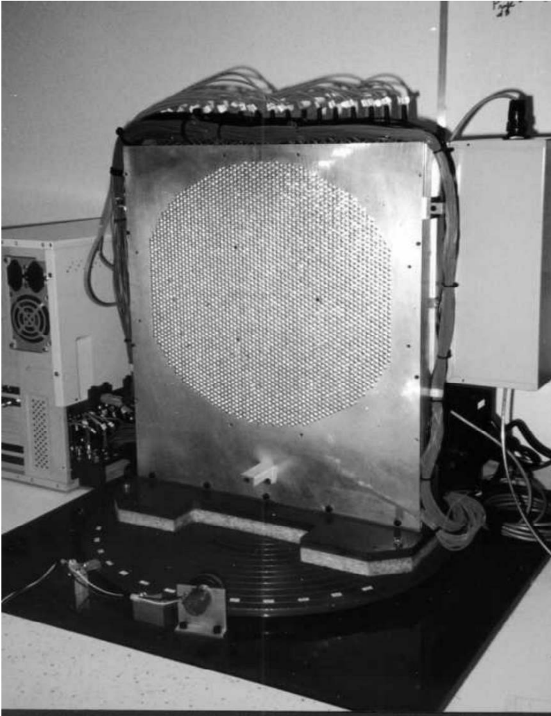
Fig. 1.31 Programmable light array of 350 mm diameter with 3046 infrared emitting LEDs (after [73] with permission by Dr. G.W.Webb)
