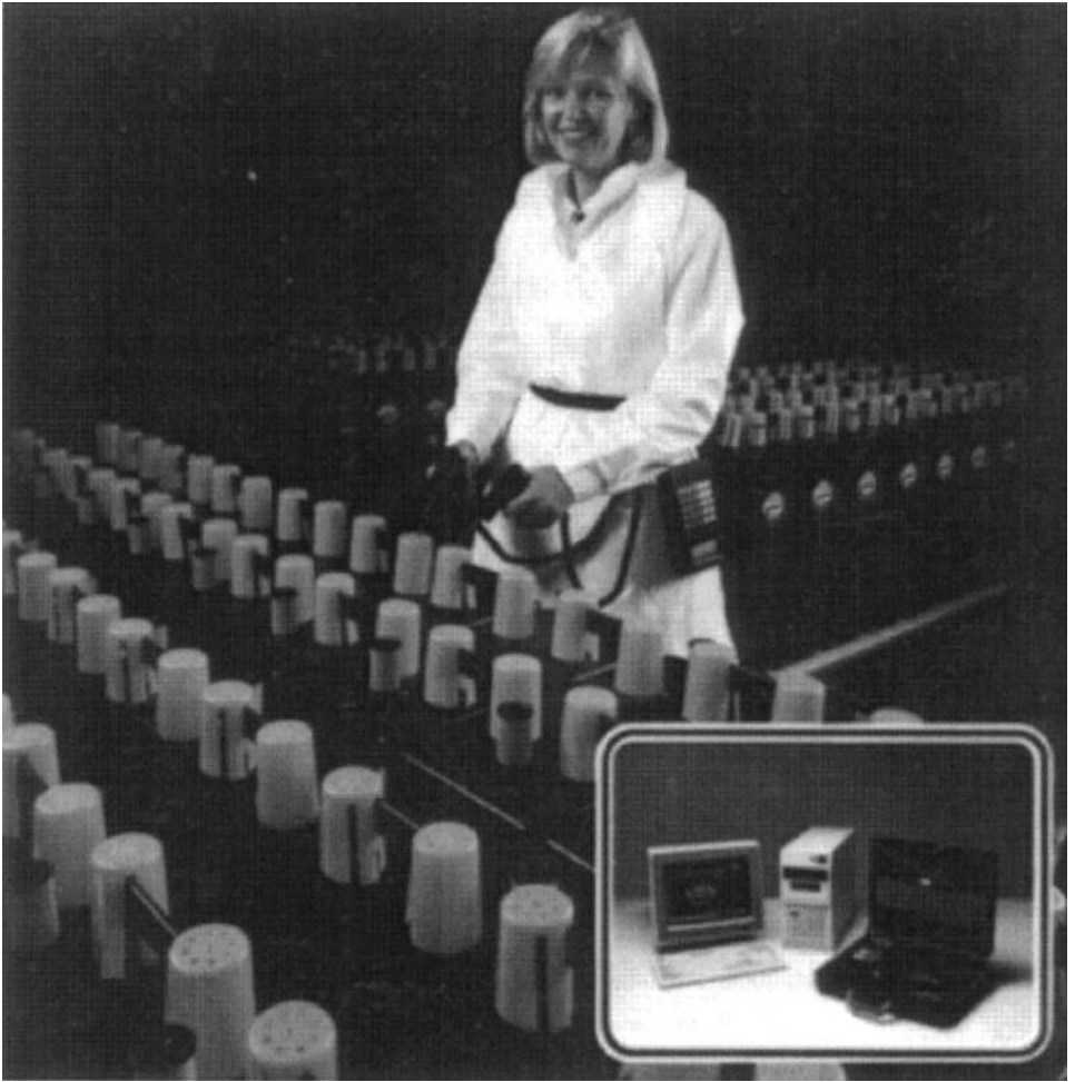
Figure 7.28 Manual service equipment that automatically registers the results and forms files that can be transferred into a PC for further processing.
