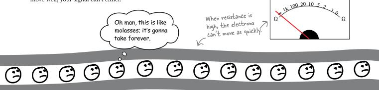
So if you're having network problems, you can use a multimeter to check out whether high resistance along the cable is slowing down your signal.
