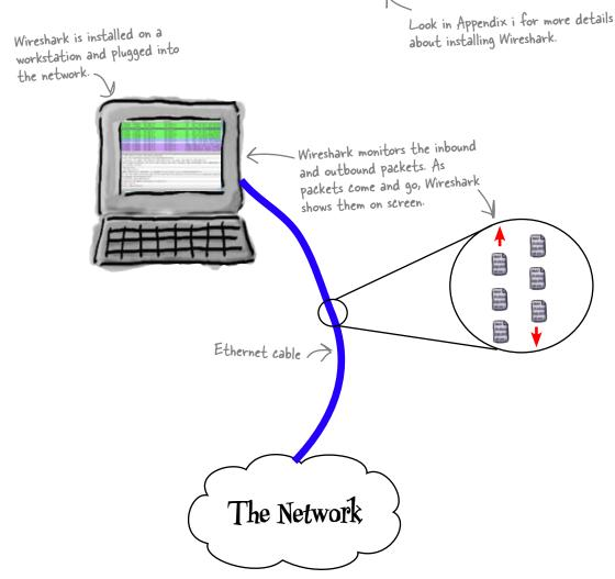
Let's use Wireshark to monitor traffic on the switch. That way we can pick up any more rogue signals the mole sends, and find out what network device sends them to the switch.
