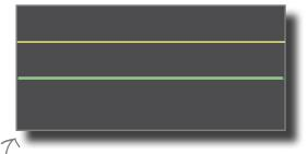
The oscilloscope shows a clear and distinct signal, but as it always falls below the logical high voltage level, the logical analyzer interprets it as a constant O.
