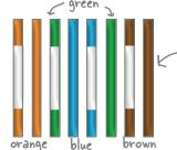
The 568B wire order is like the 568A wire order but with the position of the green and orange wires switched around.
