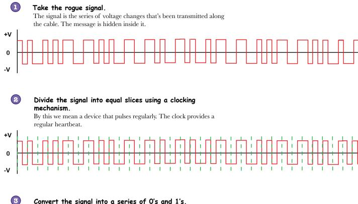
**Convert the signal into a series of O's and 1's**. To do this, look at the voltage level where the clock pulse meets the signal. The voltage level at this point determines whether the value is a 0 or a 1.
