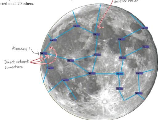
The Moonbase 1 router is able to send packets to the moonbases it's directly connected to, but it can't communicate with any of the other 18 moonbases it's only connected to indirectly.
