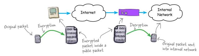
VPN works by encrypting the packets destined for the internal network. It then puts those encrypted packets into the data section of a regular TCP packet, sends that packet across the public network, and then the VPN gateway removes the encrypted packet, decodes it and sends it into the internal network.
