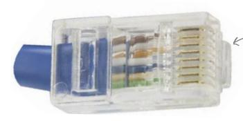
Each wire in the cable goes into a slot in the RJ-45 connector. This fixes the wire to a pin in the connector.
