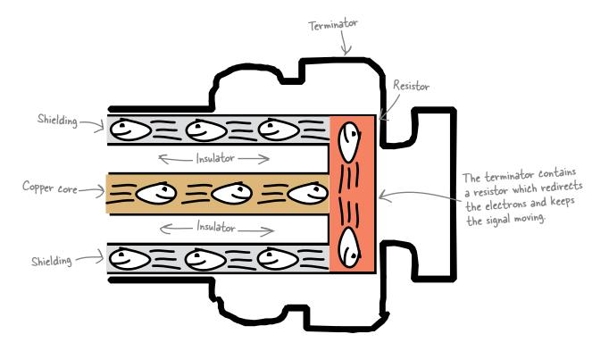
So how do we find a break in continuity in a coaxial cable network? We need to listen to electrons...
