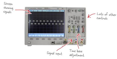
This is the same oscilloscope we saw earlier, but it can work as a logic analyzer as well. Yes, it's very expensive.
