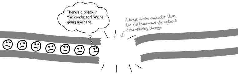
This means that if there's a break in the coaxial conductor of the bus, Coconut Airways will get network error messages.
