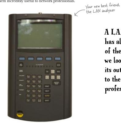
A LAN Analyzer has all the functions of the previous tools we looked at, but its output is geared to the network professional—you.
