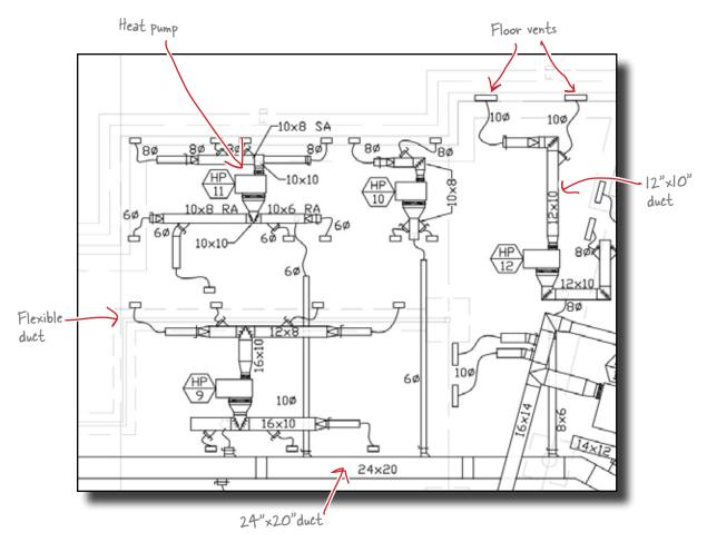
Most of this ductwork will hang via hangers from the floor joists, hanging down about 2'.
