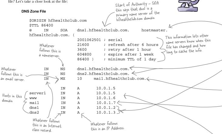
The best way to interpret this is to start reading from the bottom of the DNS zone file upwards.
