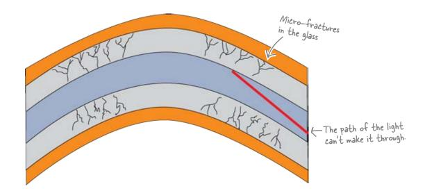
Fiber-optic cables usually have a minimum bend radius of 3.0 cm. If the cable's bent more than this, the fiber core can develop micro-fractures, real fractures, or severely leak light. And as it's the light that's carrying the network data, a loss of light means a loss of information and network errors.
