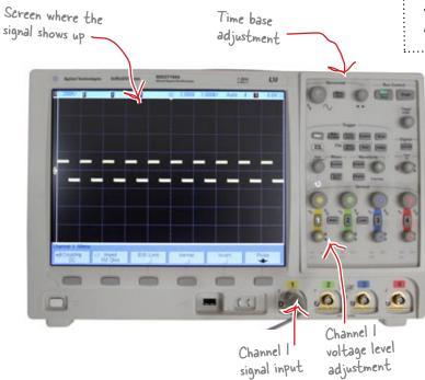
Here's an example readout from the oscilloscope showing you the voltage changes in a cable over time.
