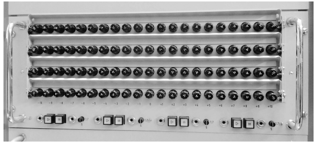
Fig. 2.25. Telefunken function generator with fixed break-points
