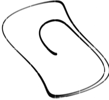
Fig. 6.23. Typical phase space plot of the solution of VAN DER POL's differential equation
