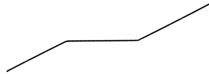
Fig. 5.27. Behavior of the dead zone circuit shown in figure 5.26
