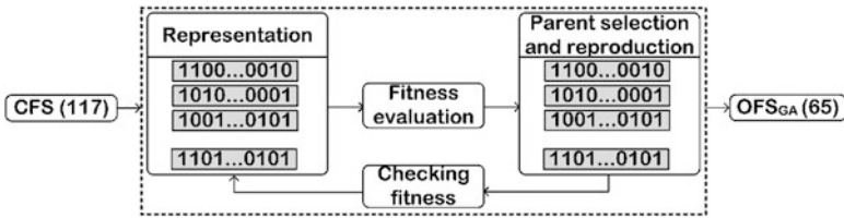
Fig. 10 General schematic for the implementation of the GA-SVM algorithm. (Note: CFS Combined feature set, OFS_{GA} Optimal feature set obtained by applying the genetic algorithm)
