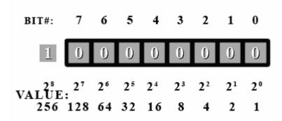
But this 9<sup>th</sup> bit (bit#8) doesn't exist. So where does it go? It actually goes into the carry bit. The carry bit, you say? The processor of the computer has an internal bit used exclusively for carry operations such as this. So if you add 1 to 255 stored in a byte, you'd get 0 with the carry bit set in the CPU. Of course, being a C++ programmer, you never get to use this bit directly. You'll need to learn assembler if you want to do that, but that's a whole other ball game.
