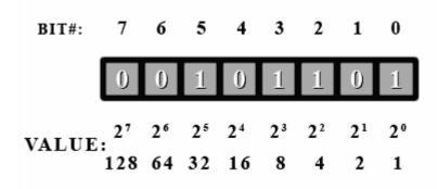
First off, we see that bit #5 is a 1, so we have  $2^5 = 32$  in our total. Next we have bit#3, so we add  $2^3 = 8$ . This gives us 40. Then next is bit#2, so 40 + 4 is 44. And finally is bit#0 to give 44 + 1 = 45. So this binary number is 45 in decimal.
