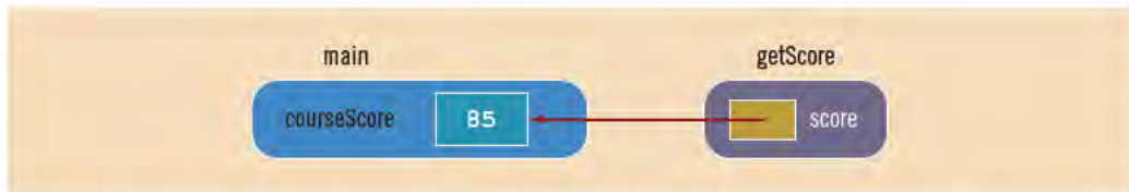
FIGURE 6-6 Variable courseScore and the parameter score after the statement in Line 16 executes
