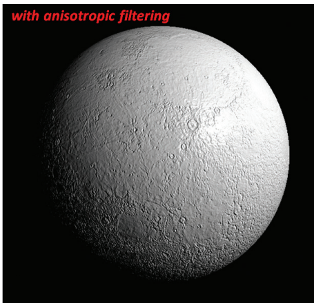
Figure 10.10 Normal mapping with AF.
