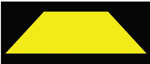
Figure 12.2 Tessellated mesh rendered with GL_FILL .
