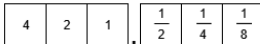
Figure 6.23 – The values that the different locations have in the binary system, to the left and right of the decimal point
