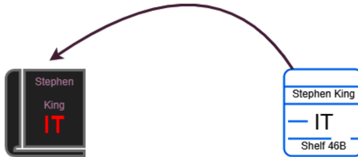
Figure 6.28 – Variables that store data by reference are like a library index card
