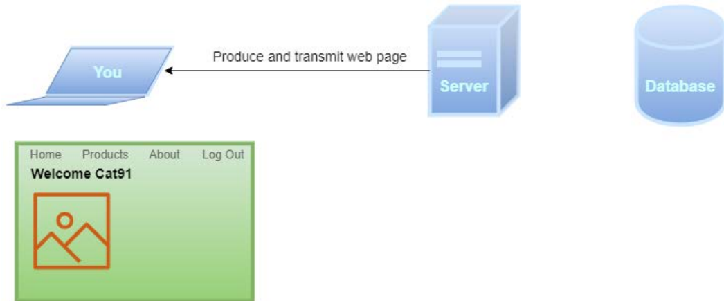
Figure 3.8 – The server produces a web page and transmits it to the client
