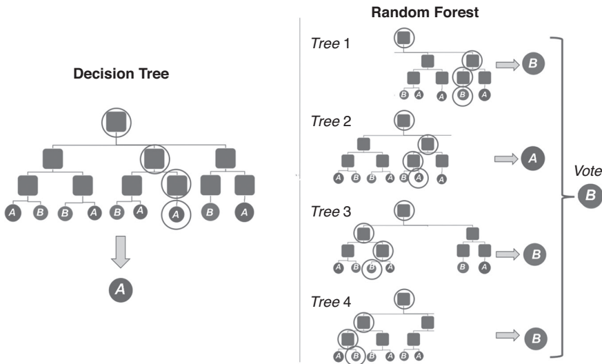
FIGURE 8.14 How a decision tree arrives at one answer, compared to random forest trees, which arrives at many answers aggregated in a voting function to arrive at a better answer when applying the decision rules to an unknown.
