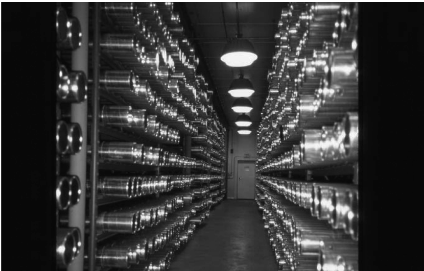
FIGURE 8.2 Ice cores inside stainless steel canisters at the National Science Foundation Ice Core Laboratory (NSF-ICL), Lakewood, Colorado. The room is kept at a constant -36^{\circ}\text{C} ( -33^{\circ}\text{F} ).
