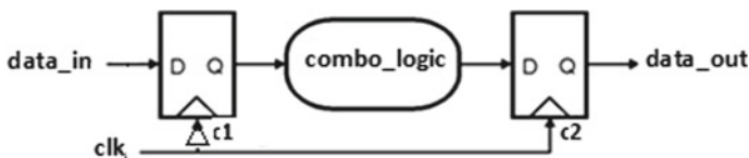
Fig. 10.15 Negative clock skew
