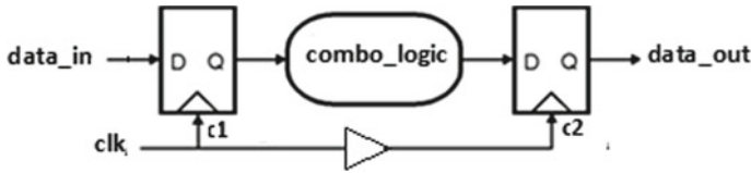
Fig. 10.14 Positive clock skew
