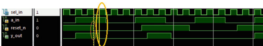
Fig. 6.21 Timing sequence for the synchronous input
