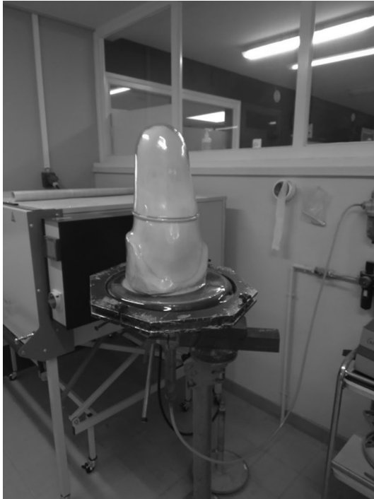
Image 1.1.3. Temporary socket in thermoplastic next to a furnace. Photograph by the author.
