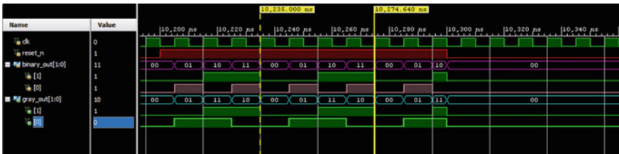
Fig. 9.7 Waveform of gray counter
