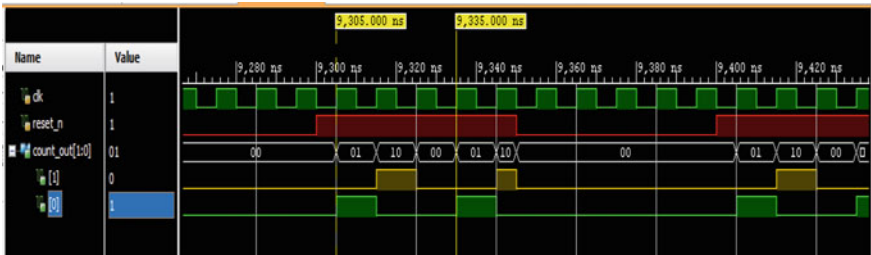
Fig. 13.7 MOD-3 up counter waveform without having 50% duty cycle
