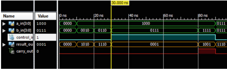
Fig. 4.7 Simulation result of 4-bit adder and subtractor
