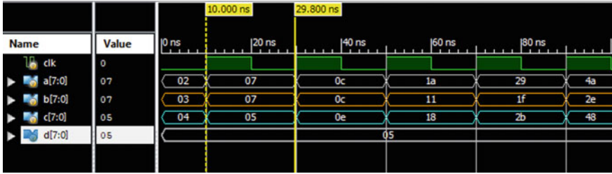
Waveform 2 Simulation result for Verilog non-blocking assignment
