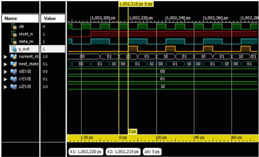
Fig. 14.20 Simulation result of FSM to detect sequence 101
