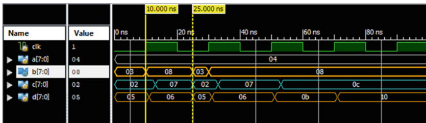
Waveform 6 Simulation result for the Verilog non-blocking assignment with intra-assignment delay
