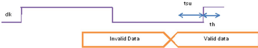
Fig. 20.2 Valid setup time region timing sequence
