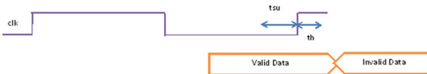
Fig. 20.3 Valid hold time region timing sequence
