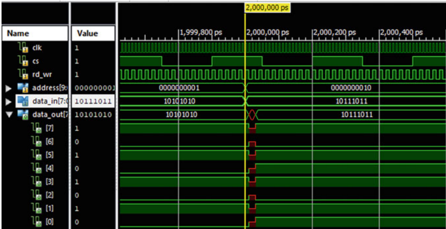
Fig. 10.13 Simulation waveform of memory
