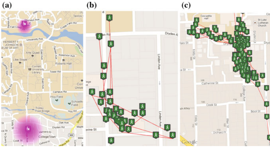
Fig. 21.1 Visualization of a user’s movements over a week a heatmap showing the locations where the user is stationary everyday b location traces of frequent walks for the user c location traces of frequent walks for another user
