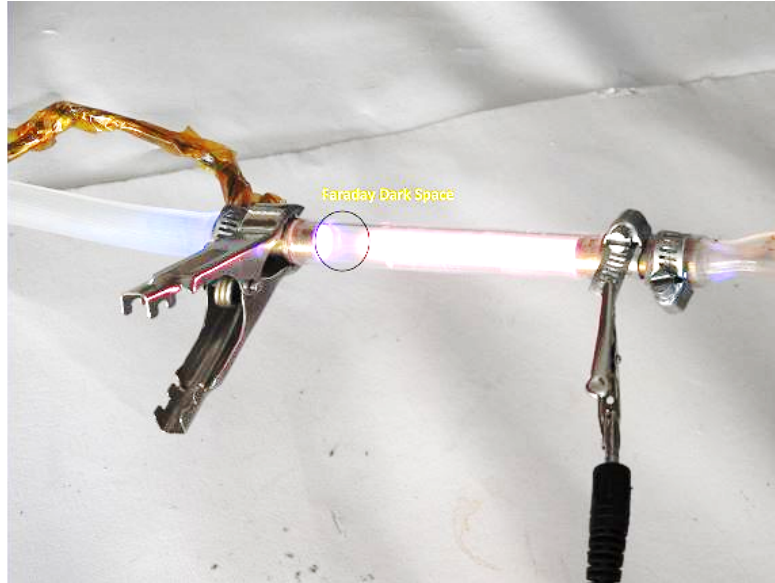
FIGURE 4.9: Experimental demonstration of DC glow discharge.
