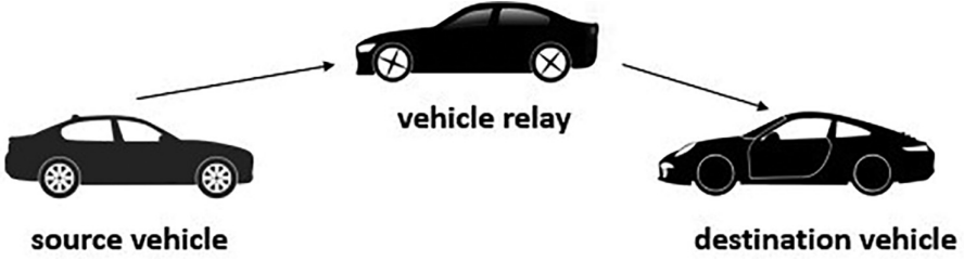
FIGURE 4.2 V2V A-F dual-hop vehicle relay communication.
