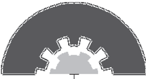
FIGURE 9.11 Half cross section of a typical 10/6 SRM with 10 stator and six rotor poles.
